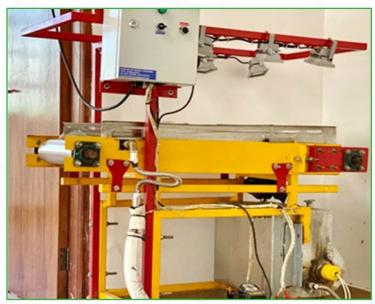
Refractance Window Drying Technology (RWDT) for production of high-quality bio-products
